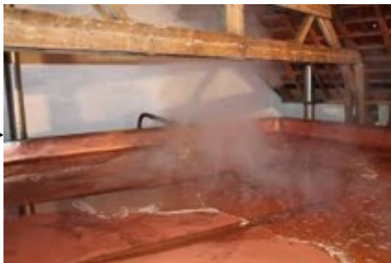
Open Air Wort Cooling
